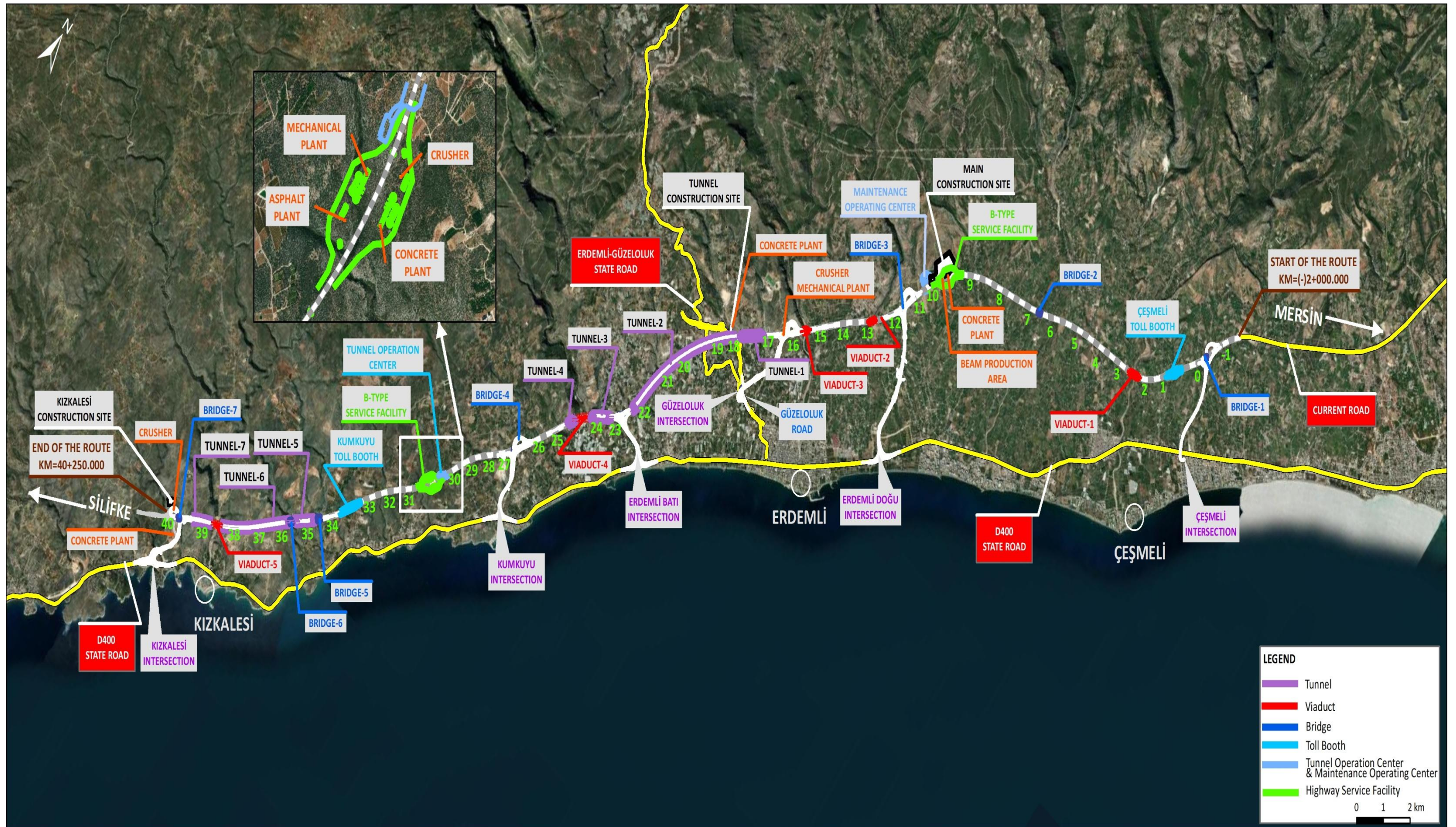
Figure 1-2 Key Components of the Project Route
